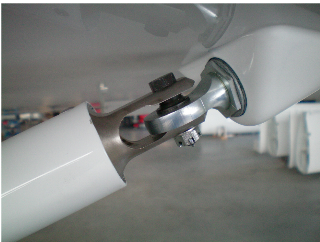
figure 2 - wrong installation of upper strut attachment with loose ball bearing
