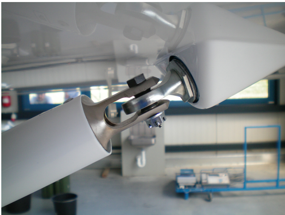
figure 1 - correct installation of upper strut attachment
