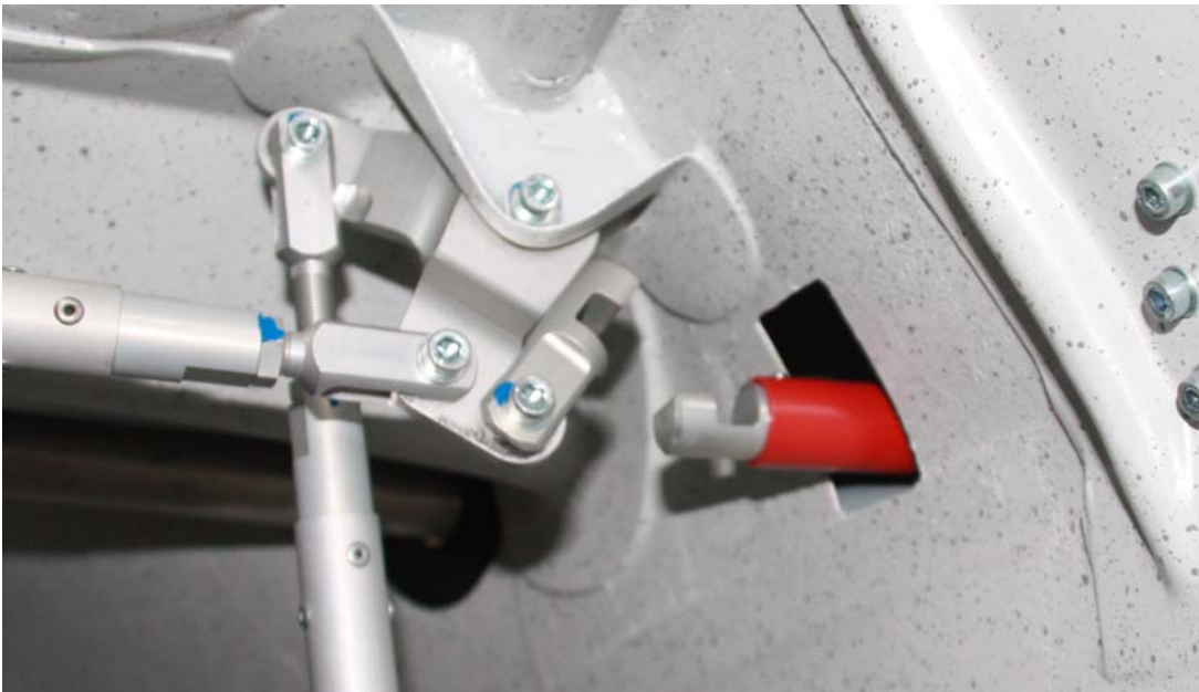
Figure 2b – opened quick- fastener
