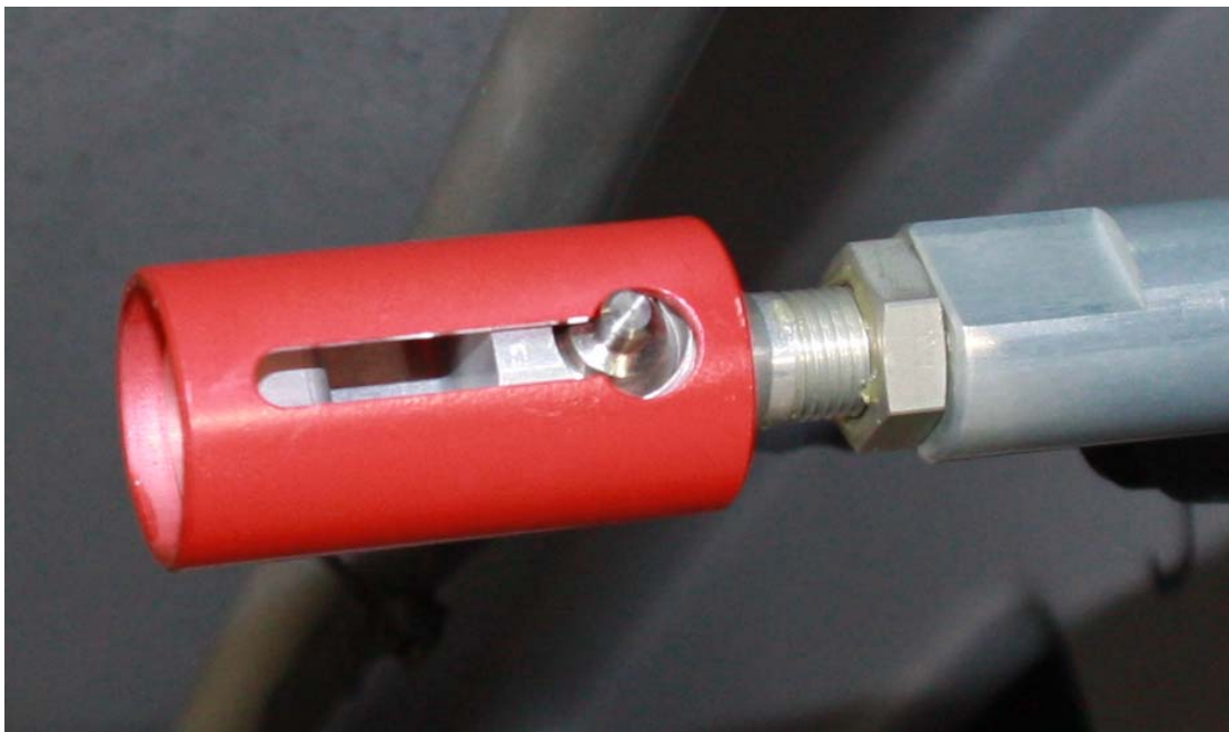
Figure 5b – insecure quick-fastener, wrong position of securing pin
