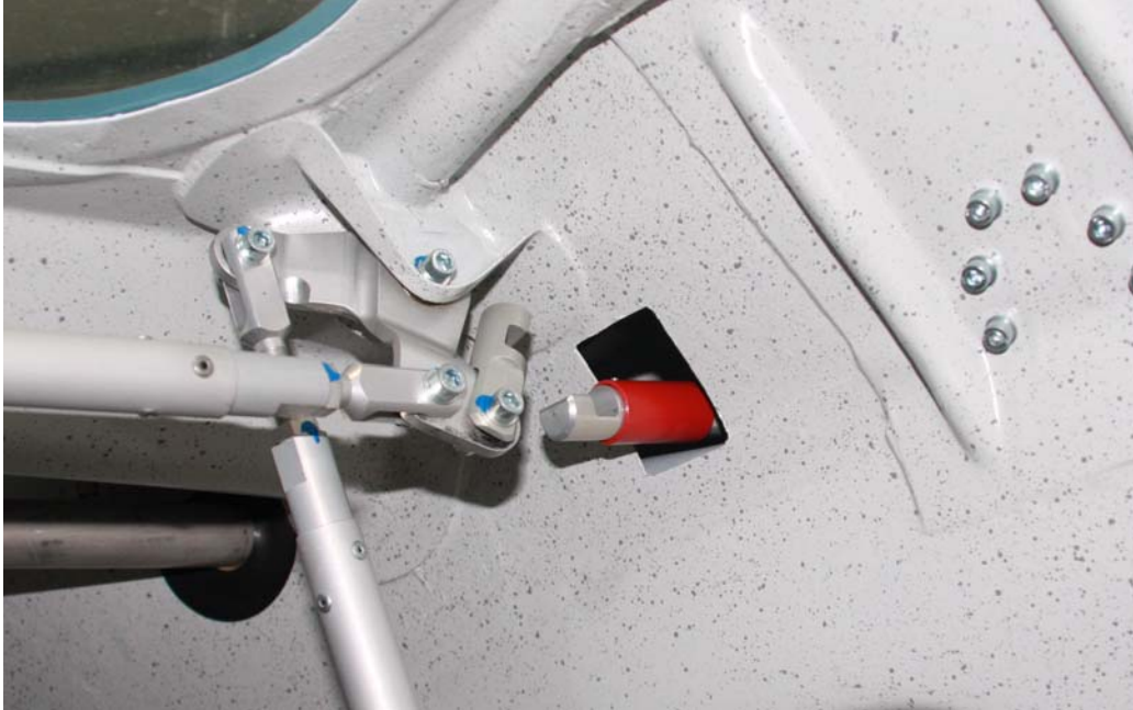
Figure 1a – port aileron quick-fastener, not connected and secured
