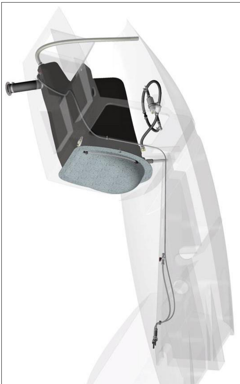
overview of airframe sided fuel system
