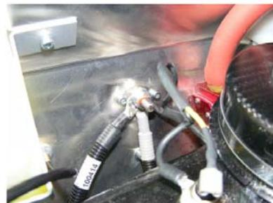
Apply LPS-3 to seal connection from atmosphere and help to prevent possible corrosion.
