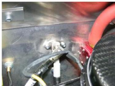
Re-assemble feed through as shown.
