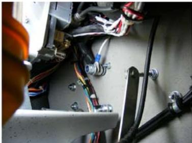
Assemble inside feed through as shown ( **do not re-install inner nut**). Torque nut to 30 Nm (266 in-lb) (22 Ft. lbs)
