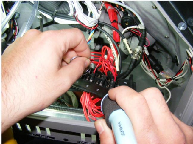
Removal of grounding stud feed through assembly.
