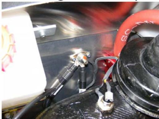
Remove nut washers and wire terminals from stud assembly.
