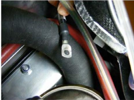
Brighten terminal ends to insure proper connection.
