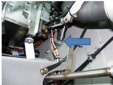
Remove self locking nut and flat washer.
