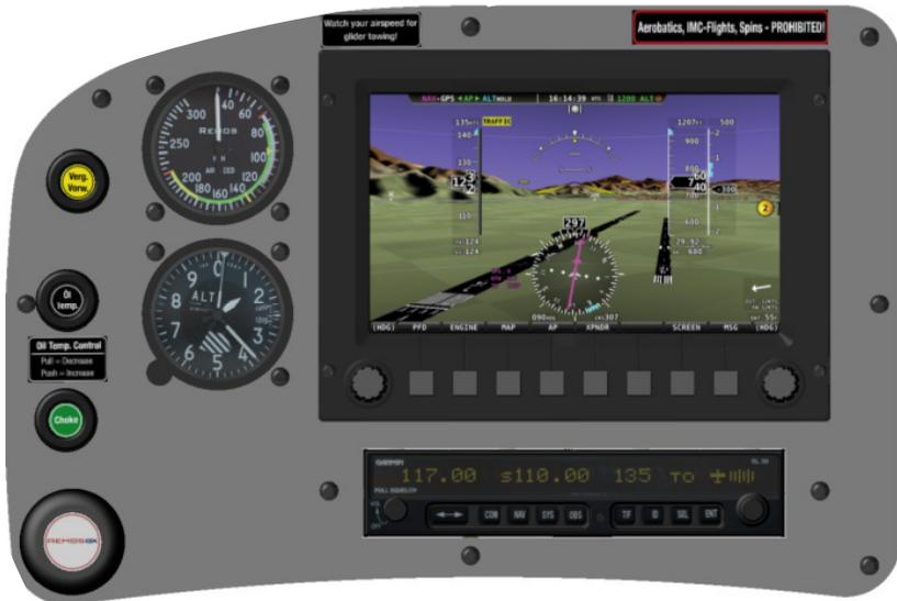
The primary flight instrumentation and the indication of the Motorparameter are carried out via the DYNON SV D700. This is a large-scale integrated advertisement system, it unites this “Electronic Flight information display and this „Multinational Function display“ what does mean all conventional primary are found here, and secondary flight instruments and navigation instruments the engine instruments on a screen again.
