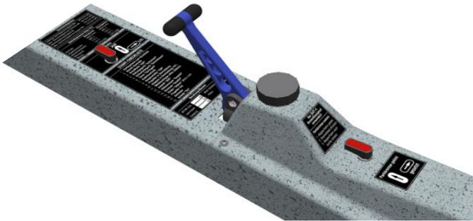
All controls are labeled. On the center console you will find all important placards, which post the operational limits for a safe operation of the aircraft. In addition a start-up checklist is provided
