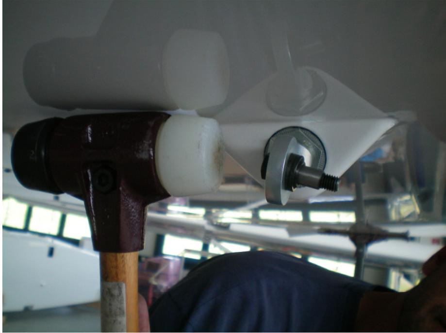
figure 1 - taking out upper ball bearing
