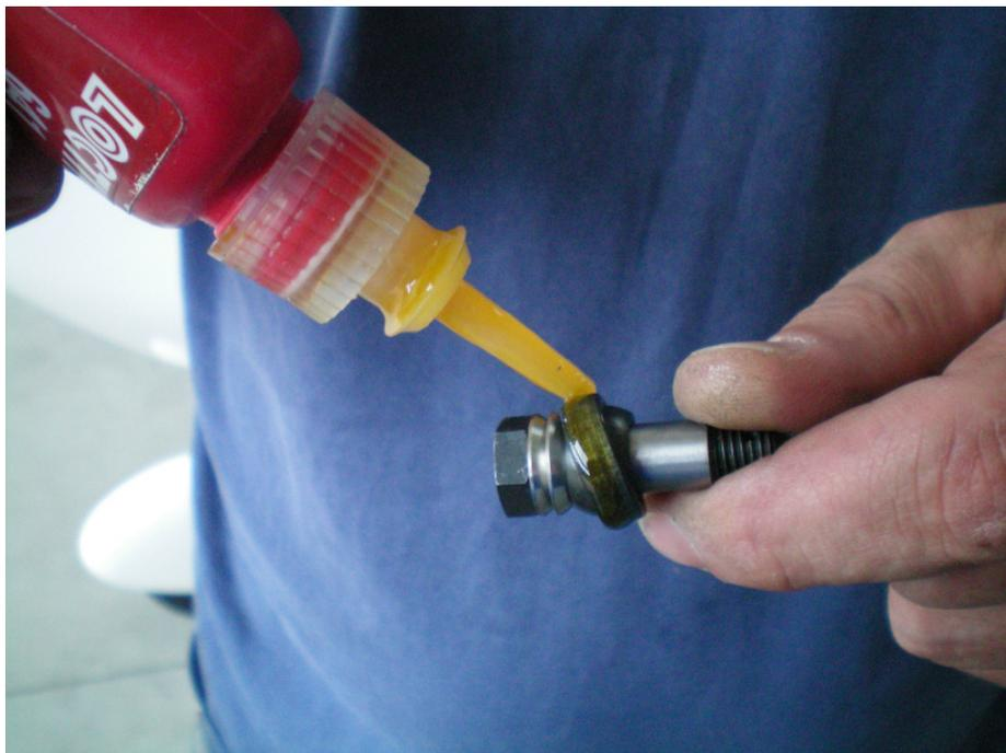
figure 2 - using Locktite 641 for glueing
