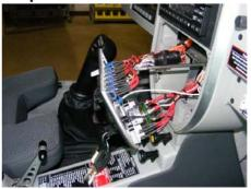
Remove 4ea. Screws from corners of panel assembly.
