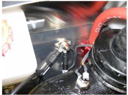
Remove nut washers and wire terminals from stud assembly. Remove attaching bolts. Remove stud assembly from airframe.
