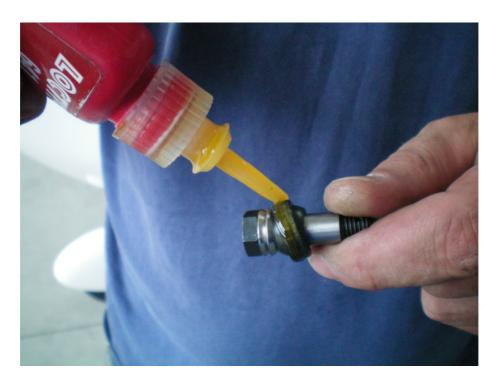
figure 2 - using Locktite 641 for glueing
