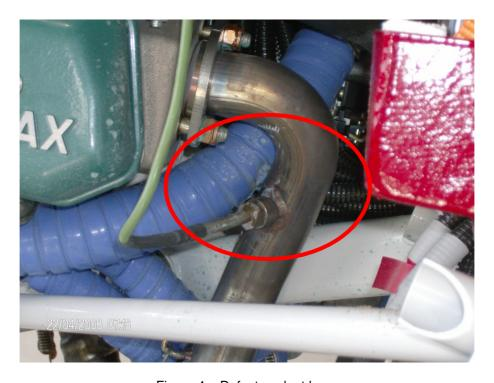
Figure 4 – Defect coolant hose
