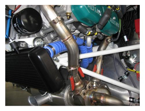
Figure 7 – Hoses from/to engine, detail view left-hand side
