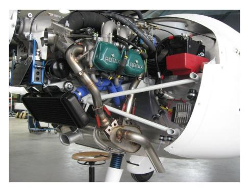
Figure 5 – Overview correct hoses from/to the engine, left-hand side
