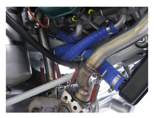
Figure 9 – Hoses from/to engine, detail view right-hand side
