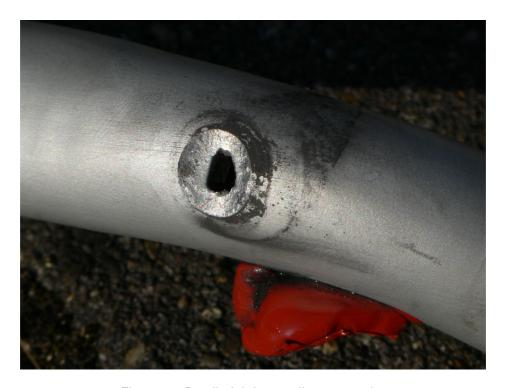
Figure 3 – Detail of defect cooling water tube
