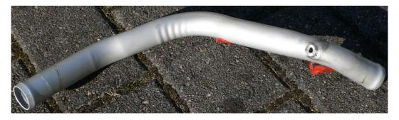
Figure 2 – Damaged cooling water tube
