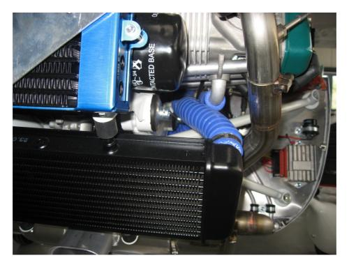
Figure 8 – Hoses from/to engine, detail view front-left
