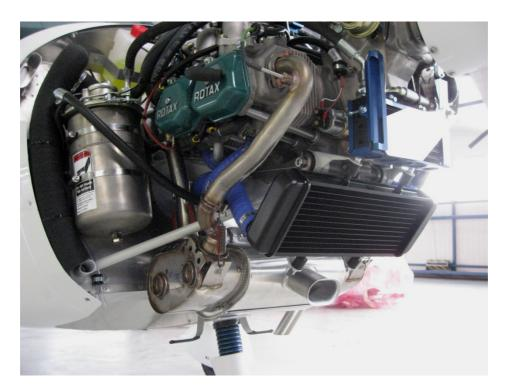
Figure 6 – Overview correct hoses from/to engine, right-hand side
