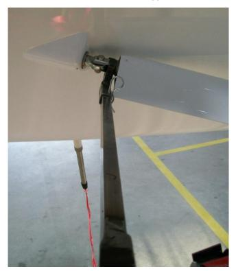
put the strut on the thread of the bracket you already attached on the fuselage, spin on nut
