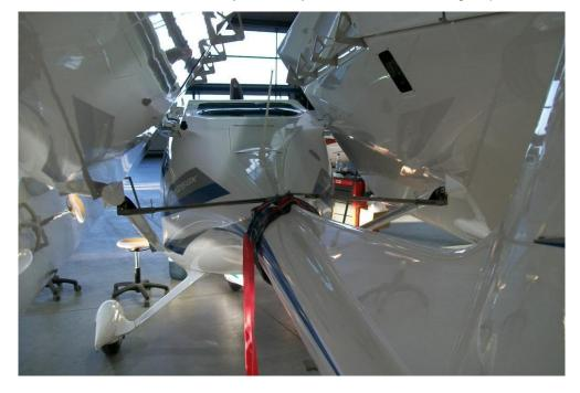
The aircraft will now sit on its tail skid. Take care not to poke the wingtips into the rudder.
