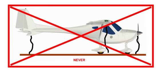
The REMOS GXiS cannot be tied down on the propeller. This rope can be omitted.
