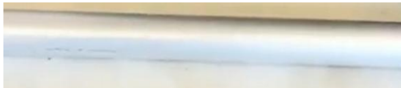
typical abrasion after app. 500h TTA
