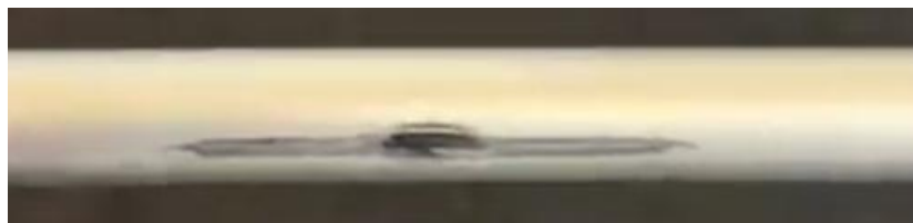
high abrasion after app. 5.000h TTA, measurement required
