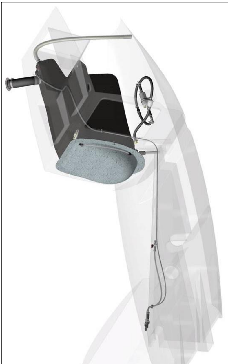
overview of airframe sided fuel system
